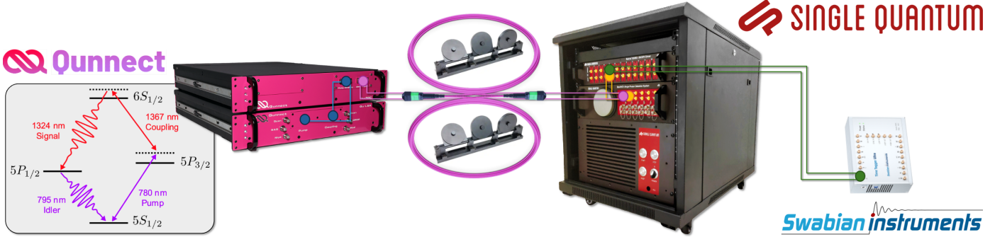
Fig. 1: Rubidium level diagram for SFWM process and schematic of measurement setup.
